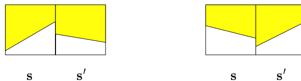
Figure 5.7: Two illustrations of the numerical problem between connected boundary cells. Only the left example causes a problem with the simplex algorithm.
